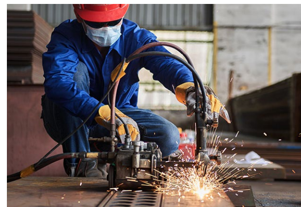
Semi-Auto Roller Gas Cut Cutting of thicker plates
