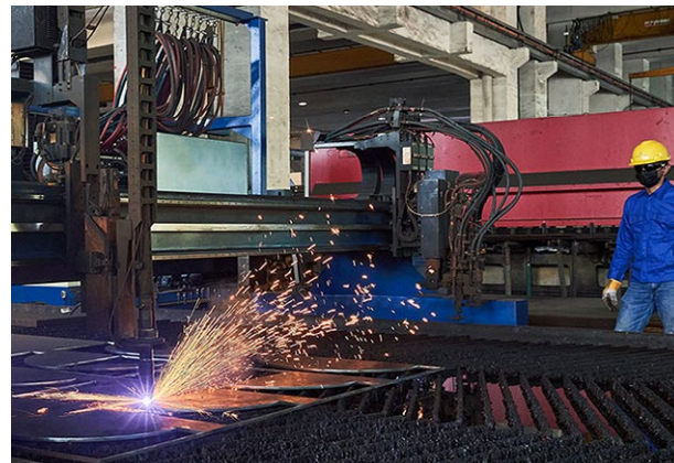
Plasma Plate Cutting Machine Cutting and drilling to desired shapes and sizes
